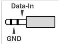
The pin connections for the 2.5mm stereo jack. The tip connector is not used.
